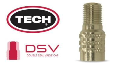
The "DSV" cap is designed to replace standard valve caps on truck and heavy-duty vehicle wheels, enabling tyre pressure to be checked and inflation to be achieved directly through the valve cap. The valve seals in the same way as a high-pressure valve cap, yet offers the convenience and simplicity of an inflate-through extension, as there is no need for the valve caps to be removed at any time.
